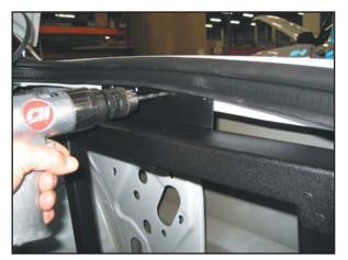
Top frame mount attachs to the trunk gasket mounting flange. Drill three holes with a 3/16" (.187") drill bit.
